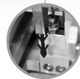
Station 4 Locking pin is placed
